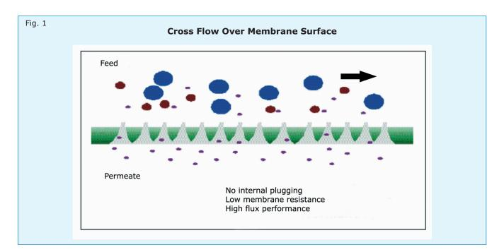
Membranes with a molecular weight cut-off (MWCO) of 100,000 remove upto 99% of non-reactive silica present in feed while
