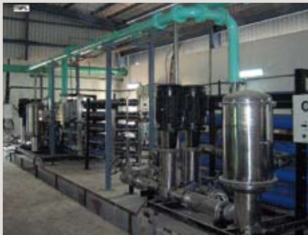
Two plants, each of 80 m 3 /h UF and RO, for Tamil Nadu Newsprint at Karur.
