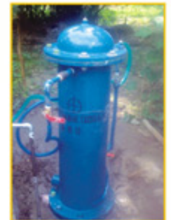
Arsenic removal hand pump attachment
