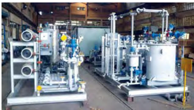
An order from Simon Carves Ltd., Saudi Arabia, for a 23.5 m 3 /h waste water treatment plant to treat fluoride-based waste
