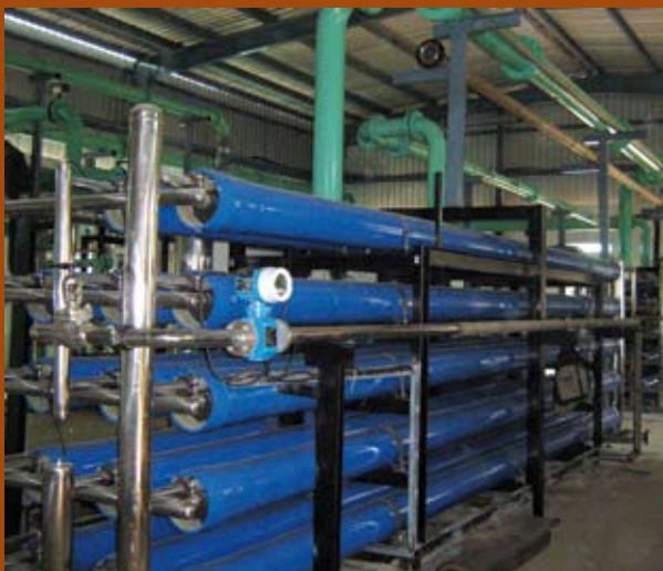
2 x 80 m 3 /h ultrafiltration and reverse osmosis plants to treat river water at Tamil Nadu Newsprint and Papers Ltd., Karur, Tamil Nadu.
