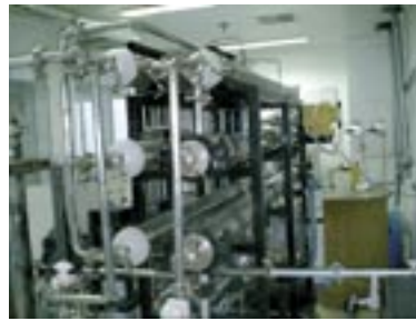
At Johnson & Johnson, Mumbai modification of competitor-supplied RO-polisher unit from 200 to 600 LPH, including addition of six SS pressure vessels and twelve HSRO membranes.
